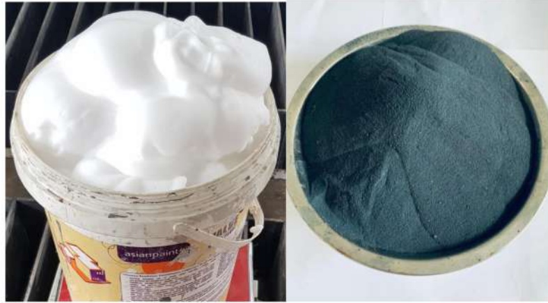
Figure 3. CLC design mix material (a) foam (b) silica fume
